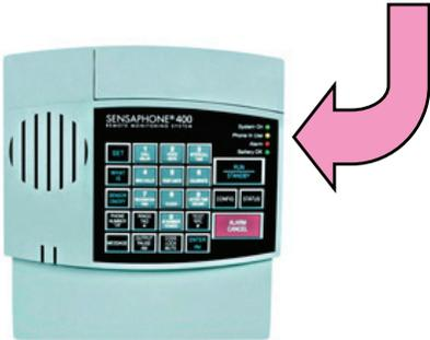
The Autodialer will respond to an alarm by dialing up to four separate telephone numbers. When the call is answered, an "Alert Condition" message is delivered and a user-recordable voice message. The Dial out sequence can be "acknowledged" by sending "555" from the phone keypad during a received call. This ceases dial out.
