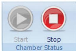
When the Chamber is running the "Stop" icon is illuminated.
