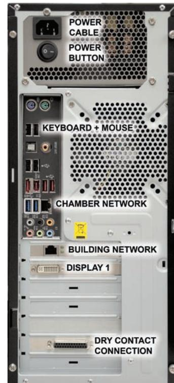
Figure 6.7: Central Management™ PC Connections
